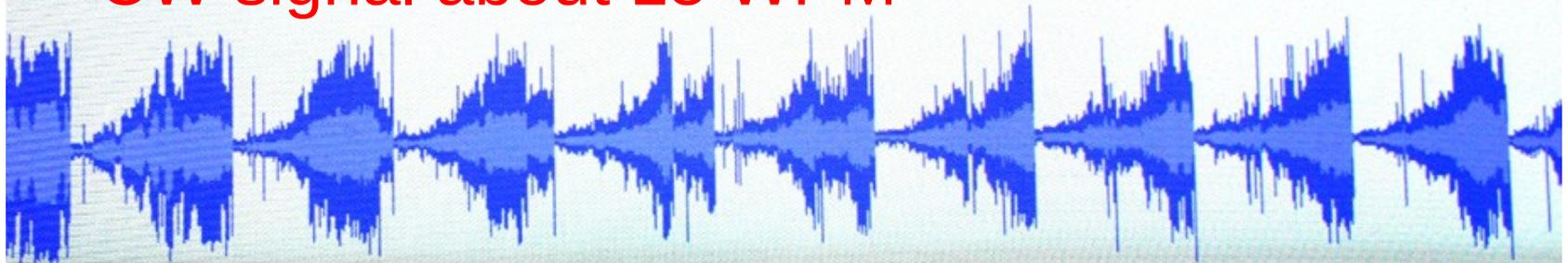
Electric Fence firing off every 2 seconds, 160 meters
