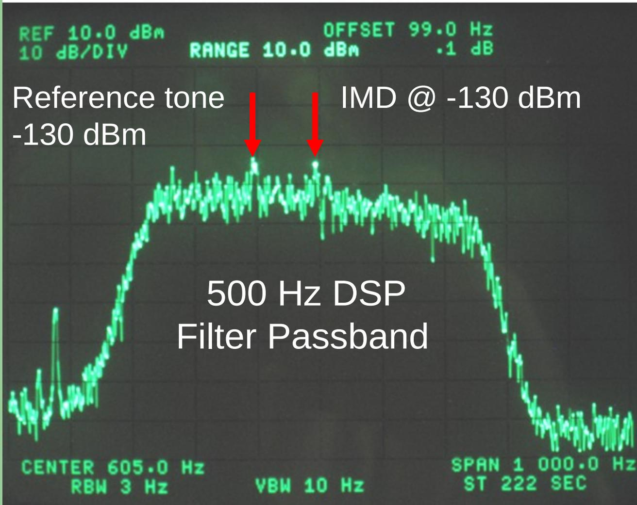
Phase noise limited dynamic range is **78 dB** at 2 kHz.
