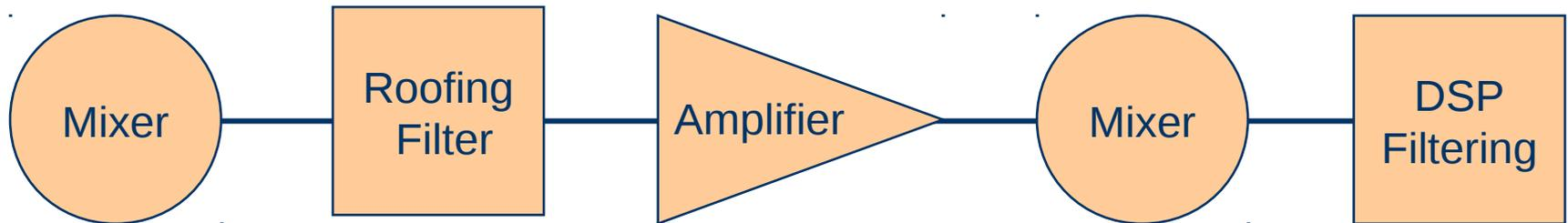
On CW, the wider the roofing filter, the worse the problem. The more signals inside the roofing filter, the more the DSP filtering is stressed. Example: The IC-7600 has a roofing filter that is about 1/3<sup>rd</sup> the width of the Pro III, and a stronger front end.
